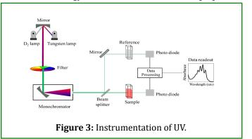
Copyright information for Figure 4: Schematic illustration of UV-Vis spectrophotometer (Source: Kumar et al. 2019 with permission from Elsevier)
