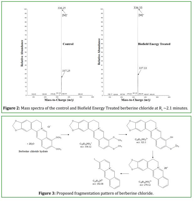
The LC-MS spectra of both the samples of berberine chloride showed the mass of the molecular ion peak at m/z 336.3 [M]<sup>+</sup> (calculated for C<sub>20</sub>H<sub>18</sub>NO<sub>4</sub><sup>+</sup>, 336.12) with 100% relative intensity. The theoretical calculation of P<sub>M+1</sub> for berberine chloride was presented as below:
