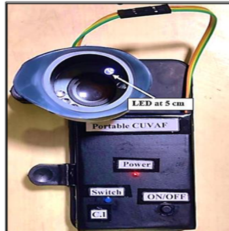
Figure 1: Shows custom developed smartphone-based conjunctival ultraviolet autofluorescence photography system used to measure the conjunctival damage.
