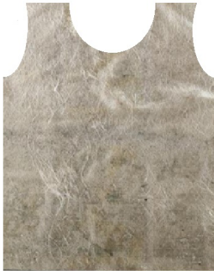
Figure 3: Inner Armour Prepared using Fiberglass Material.
