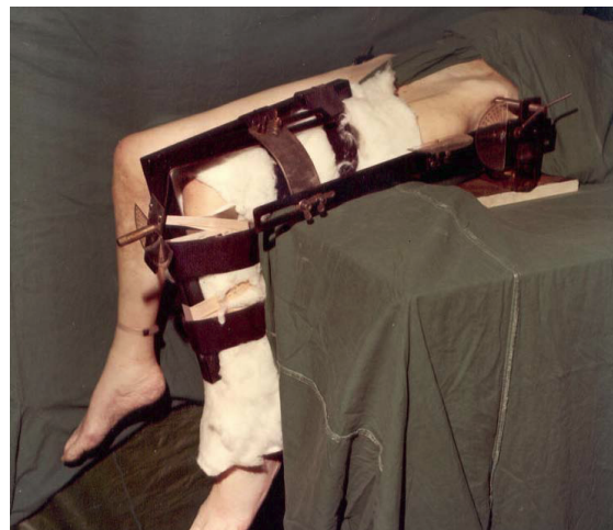
Figure 2: Device used to test stability of the hip joint showing pelvis fixed and protactors to measure the angle of flexion/extension, adduction/abduction and internal/external rotations (Courtesy: Photograph reproduced with the kind permission of Injury/Elsevier).
