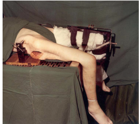
Figure 1: Device used to test stability of the hip joint showing pelvis fixed and protactors to measure the angle of flexion/extension, adduction/abduction and internal/external rotations (Courtesy: Photograph reproduced with the kind permission of Injury/Elsevier).
