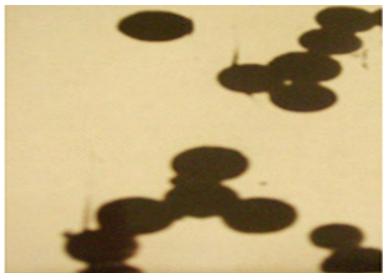
Figure 4: Electron microscopic photograph of polystyrene latex obtained after 6 hours withstanding of static system.
