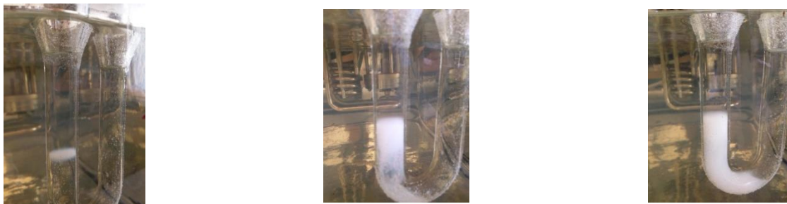
Figure 4: Dynamics of latex in static system vinyl acetate - aqueous solution of potassium persulfate in the presence of methanol.
