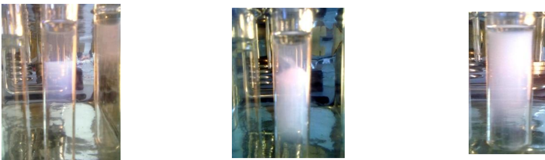
Figure 3: Dynamics of latex formation in static system styrene - aqueous solution of potassium per sulfate in the presence of methanol.
