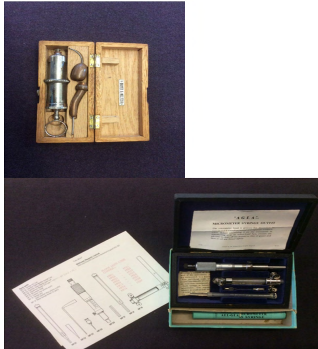
Figure 6: Top is the copper cased cannulas and the thick metal syringe with a robust screw lock retain heat to enable the injection of melted paraffin wax into hollow organs and vessels for demonstration specimens for morbid anatomy classes.
